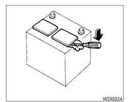
Remove the vent caps with a screwdriver as shown. Use a cloth to protect the battery case.
